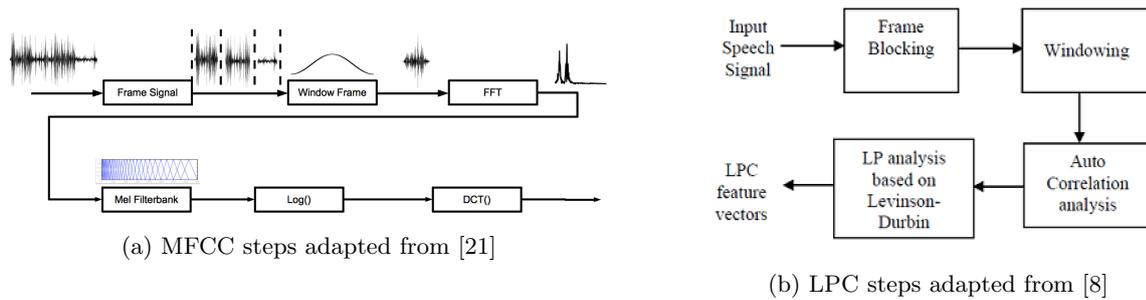
Figure 4: Features extraction from sound signals
